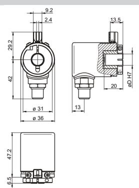
With flange connector M12 and torque pin
