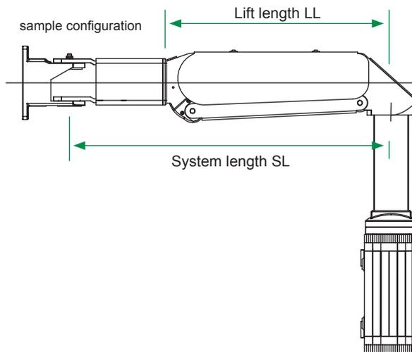
**System length: SL** \_\_\_\_\_ mm
